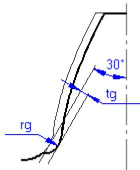
$Y_\delta$  ... notch sensitivity factor (depends on the material and curvature radius of dedendum transition)
