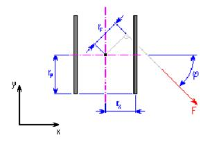
In any weld point, a common force F causes adequate stress to the stress which would arise by combined loading from bending moment  $M_F$  and the pair of shearing forces  $F_X$ ',  $F_Y$ ' with action point in the weld group center of gravity, while applies:
