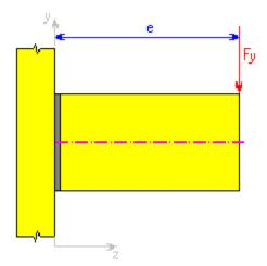
For calculation purposes, the bending force can be substituted by the combination of shearing force  $F_{Y}$  acting in the weld plane and the bending moment M acting in the plane perpendicular to the weld plane. Then the stress in the weld can be calculated using the previously mentioned procedure.
