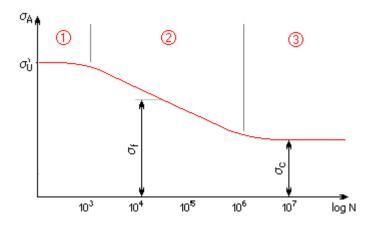
If the weld joint is calculated on the condition of finite life in the area of timed strength, the finite-life fatigue limit  $\sigma_f$  or  $\tau_f$  must be known for determining the joint strength. An empirical formula  $\sigma_f = 10^{Y} N_X$  is used for calculation of this limit if the endurance limit se is known. Exponents are calculated according to:
