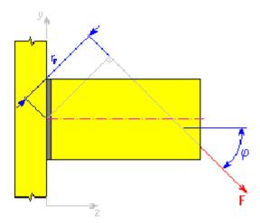
For calculation purposes, the common force F can be substituted by the combination of shearing force  $F_{\rm Y}$  acting in the weld plane with the axial force  $F_{\rm Z}$  and the bending moment M acting in the plane perpendicular to the weld plane. Then the stress in the weld for so defined loading can be calculated using the above mentioned procedure.
