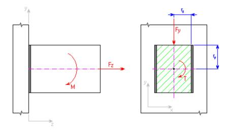
Loading in the plane perpendicular to the weld plane induces a tensile or pressure stress  $\sigma$  in the weld.
