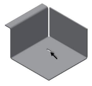
**Note:** If the slot is not oriented as shown in figure, then click the **Geometry** tab on the **PunchTool** dialog and type-in **90** in the **Angle** box.
