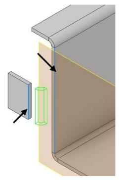
7. Make sure the **Bend Extension** is set to perpendicular.
