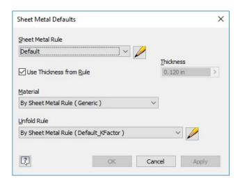
This dialog displays the default preferences of the sheet metal part such as sheet metal rule, thickness, material, and unfold rule. You can change these preferences as per your requirement.
