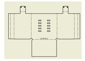
12. Likewise, select other bend lines on the flat pattern. You can also drag a selection box to select all the bend lines from the flat pattern view.
