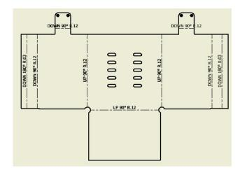
13. To add centerlines to the flat pattern view, click the right mouse button on it and select **Automated Centerlines**.
