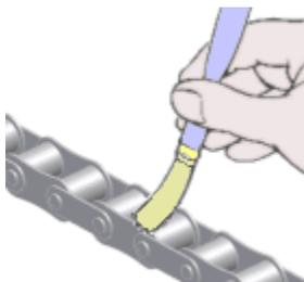
*Manual lubrication:* Oil is applied copiously with a brush or spout can at least once every 8 hours of operation. The drive is stopped and power to the drive is locked out. Volume and frequency should be sufficient to prevent overheating of the chain or red-brown (rust) discoloration in the chain joints.
