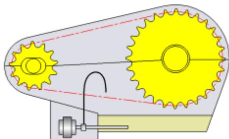
*Forced feed lubrication:* The lubricant is supplied by a circulating pump capable of supplying chain drive with a continuous stream of oil. The oil should be directed at the slack strand and applied inside the chain loop and evenly across the chain width to ensure that the oil reaches all bearing surfaces. An oil cooler and oil filter can be used if necessary.
