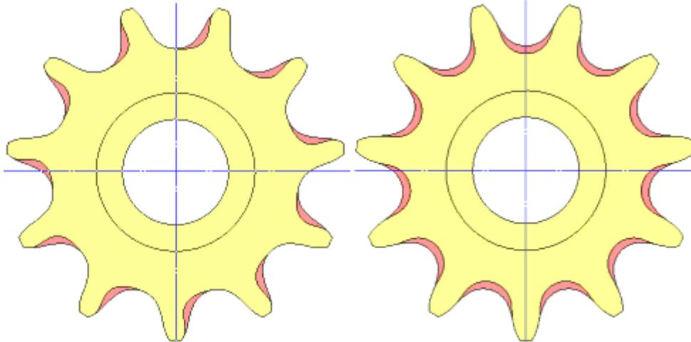
Worn roller chain drive sprocket
