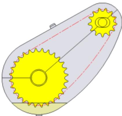
*Bath lubrication:* The lower strand of chain runs through a sump of oil in the drive housing. The oil level should reach the pitch line of the chain at its lowest point while operating.
