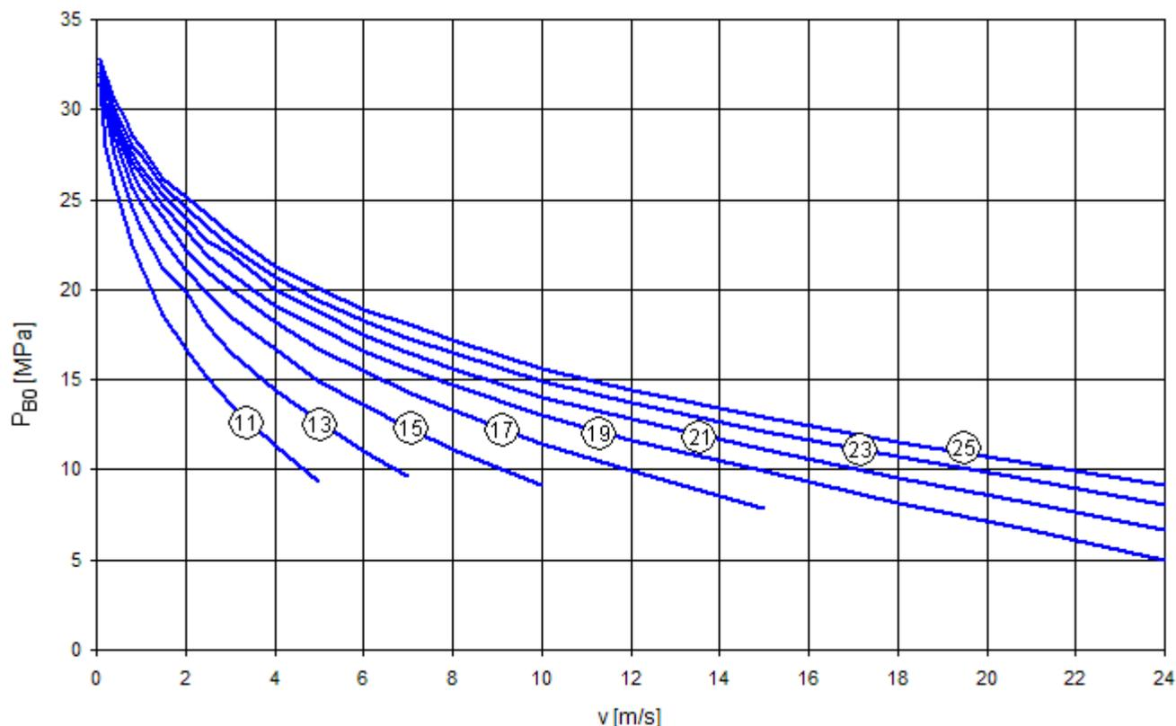
The permissible pressure obtained from the previous chart is also corrected by chain construction factor so the amount of permissible pressure is defined as follows
