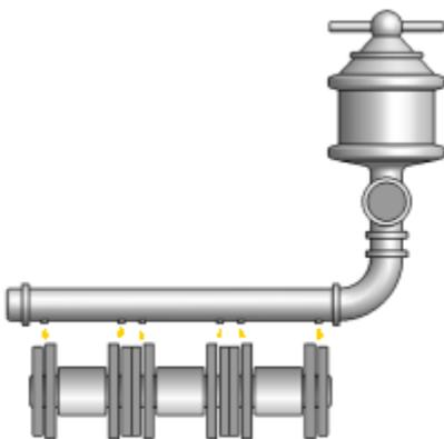
*Drip lubrication:* Oil continuously dripped onto the upper edges of the link plates, or sidebars, from a drip lubricator. Volume and frequency should be sufficient to prevent red-brown (rust) discoloration of lubricant in the chain joints. Usually the drip rate is from 4 to 20 or more drops per minute. Precaution must be taken against misdirection of the drops by windage.
