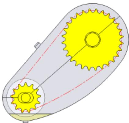
*Disc lubrication:* The chain operates above the oil level. The disc picks up oil from the sump and deposits it onto the chain, usually with a through. The diameter of the disc should be such as to produce adequate rim speed to pick up oil effectively. Higher speeds can cause oil foaming and overheating.
