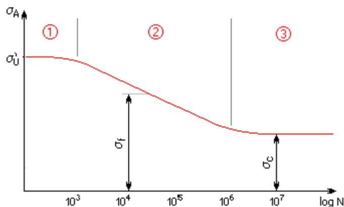
If the weld joint is calculated on the condition of finite life in the area of timed strength, the finite-life fatigue limit  $\sigma_f$  or  $\tau_f$  must be known for determining the joint strength. An empirical formula  $\sigma_f = 10^Y N^X$  is used for calculation of this limit if the endurance limit  $\sigma_e$  is known. Exponents are calculated according to:
