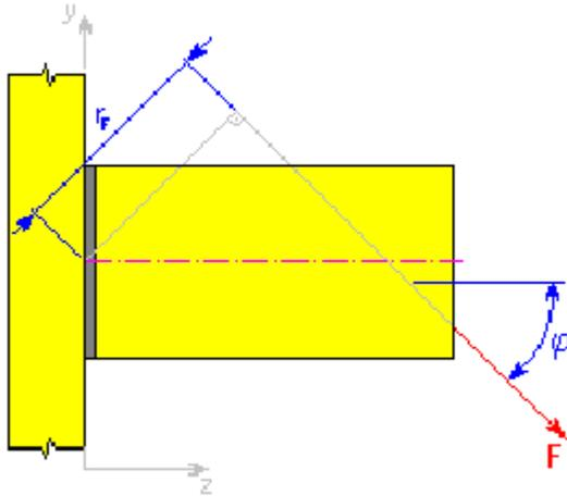
For calculation purposes, the common force  $F$  can be substituted by the combination of shearing force  $F_Y$  acting in the weld plane with the axial force  $F_Z$  and the bending moment  $M$  acting in the plane perpendicular to the weld plane. Then the stress in the weld for so defined loading can be calculated using the above mentioned procedure.
