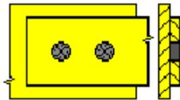
Shear stress in the weld base area
