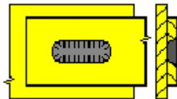
Shear stress in the weld base area
