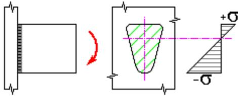
The maximum stress is originated in the outer points of the weld group, the most distant places from the neutral axis. For welds, symmetrical along the neutral axis the size of these stresses is identical. For nonsymmetrical welds, pressure stress might be greater. Normally the program tests a greater value from these peaks during strength check, regardless of the stress direction, which is pressure stress in this case.
