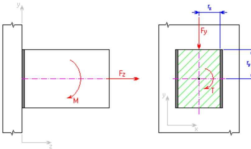
Loading in the plane perpendicular to the weld plane induces a tensile or pressure stress  $\sigma$  in the weld.
