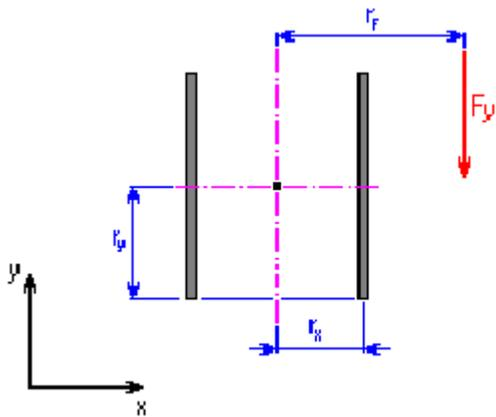
In any weld point, a stress caused by shearing force  $F_Y$  and bending moment  $M_F$  originates. Its size determines the formula:
