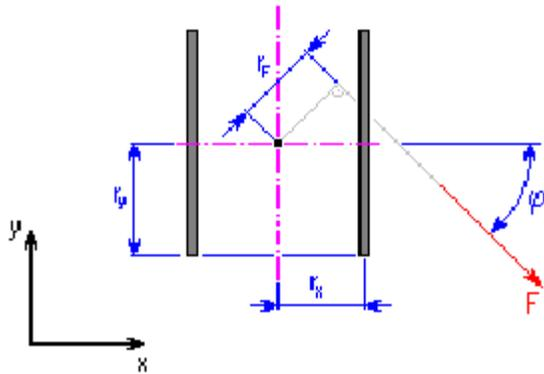
In any weld point, a common force  $F$  causes adequate stress to the stress which would arise by combined loading from bending moment  $M_F$  and the pair of shearing forces  $F_{X'}$ ,  $F_{Y'}$  with action point in the weld group center of gravity, while applies:
