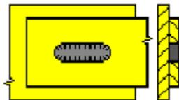
Shear stress in the weld base area
