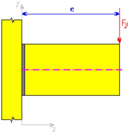
For calculation purposes, the bending force can be substituted by the combination of shearing force  $F_Y$  acting in the weld plane and the bending moment  $M$  acting in the plane perpendicular to the weld plane. Then the stress in the weld can be calculated using the previously mentioned procedure.
