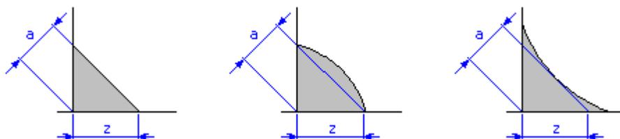
The size of fillet weld height approximately specifies the  $a = 0.7z$  formula, where  $z$  is the fillet weld width. Minimum fillet weld height is selected according to the thickness of the thicker welded part and according to the material. The following table presents the values of the recommended minimum fillet weld height.
